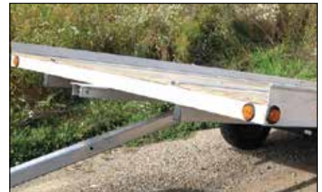
Heavy Duty tongue with guide improves turning radius
